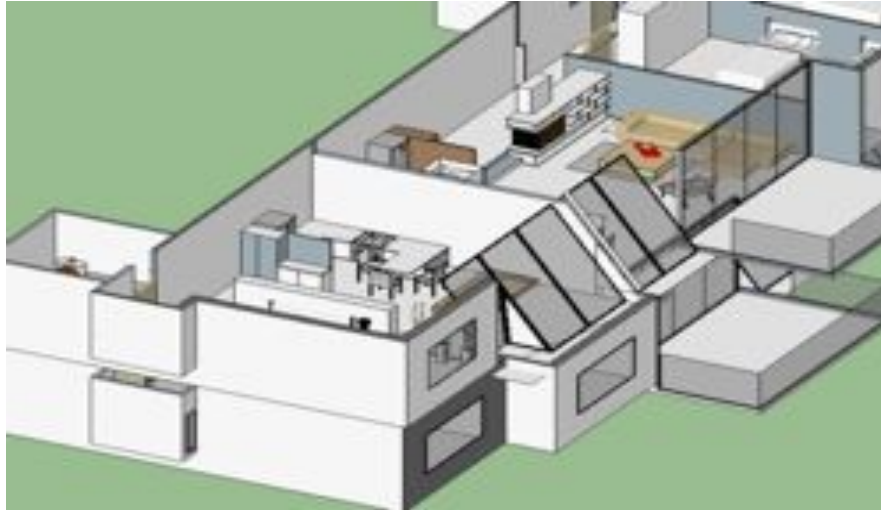
Figure 13. Transparent surfaces of living areas placed at an angle of 63^{\circ} due to the sun's rays in south direction do 27^{\circ} angle to the earth.
